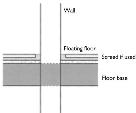
If the wall is a sound resisting or internal solid wall, with an average mass of less than 355 kg/m<sup>2</sup> (including any plaster finishes), the floor base including any structural screed should pass through.
