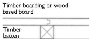
Timber boarding or wood based boards should be at least 18 mm thick and have tongued and grooved edges. Fix to 45 mm x 45 mm battens so that the nails do not go through the batten (to maintain isolation). Raft should be laid loose on a resilient layer.
