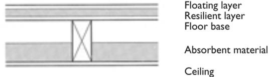
Floating layer of at least 18 mm thick timber or wood-based board with tongue and grooved edges with all joints glued and spot bonded to substrate of at least 19 mm thick plasterboard, or material with at least the same mass, on resilient layer of at least 25 mm thick mineral fibre, density 60-80 kg/m<sup>3</sup>.
