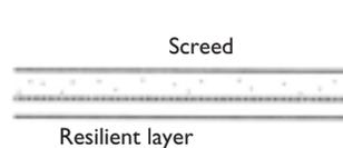
65 mm cement sand screed with mesh underlay to protect the resilient layer while the screed is being laid.
