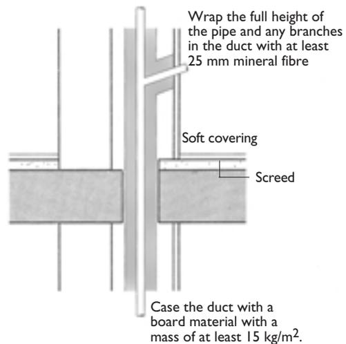
Penetrations through a separating floor by ducts and pipes should also have fire protection in accordance with Technical Guidance Document B. Rigid contact between pipe and floor should be avoided.
