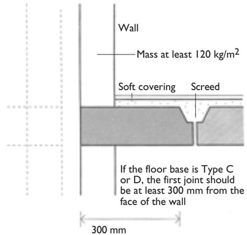
Where the floor meets an external wall or a cavity separating wall, the floor base and any structural screed should pass through whether it spans parallel with or at right angles to the wall. The cavity should not be bridged.
