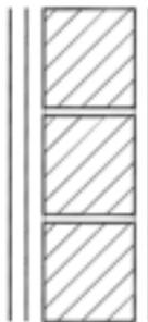
The average mass (including plaster and plasterboard) should be at least 415 kg/m<sup>2</sup>. 12.5 mm plasterboard dry-lining attached directly to plaster (no cavity or air gaps). Use blocks which extend to the full thickness of the wall.
