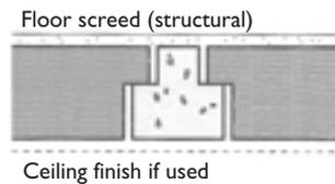
The average mass of the base (including the blocks if they are clay or concrete, floor screed, and any ceiling finish bonded to the beams or blocks) should be at least 220 kg/m<sup>2</sup>.
