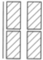
The width of the cavity should be at least 50 mm.
