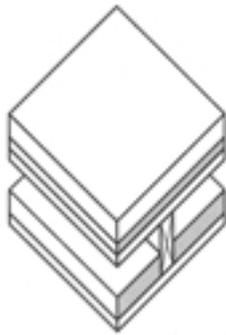
This type of floor is similar in concept to Floor Type 2 but the construction is entirely of timber.
