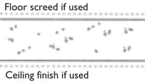
The average mass of the base (including floor screed and any ceiling finish bonded to the concrete) should be at least 220 kg/m<sup>2</sup>.
