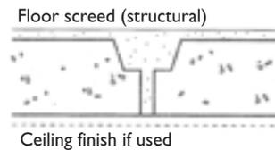
The average mass of the base (including floor screed, and any ceiling finish bonded to the beams) should be at least 220 kg/m<sup>2</sup>.
