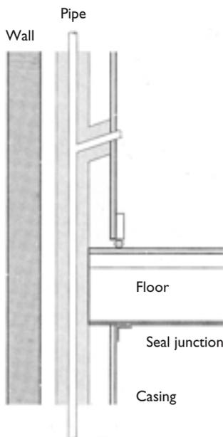
Wrap the full height of the pipe and any branches in the duct with at least 25 mm unfaced mineral wool.
