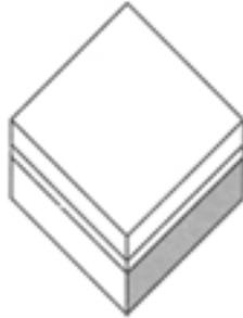
The resistance to airborne sound depends mainly on the mass of the concrete base and partly on the mass of the floating layer.
