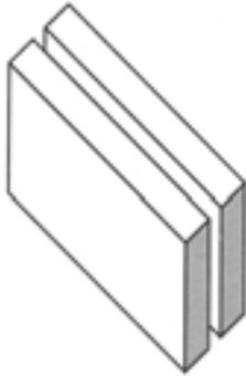
The resistance to airborne sound depends mainly on the mass of the leaves and the degree of isolation provided. In general, a cavity wall does not perform better than a solid wall of similar materials and mass.
