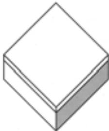
The resistance to airborne sound depends on the mass of the concrete base. The soft covering reduces the impact sound at source.
