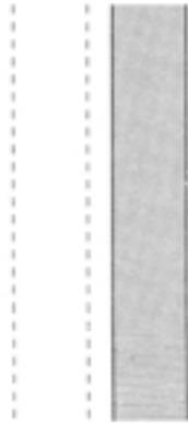
The average mass of the external wall (or inner leaf of cavity wall) should be at least 120 kg/m<sup>2</sup> (including any plaster but not dry lining).
