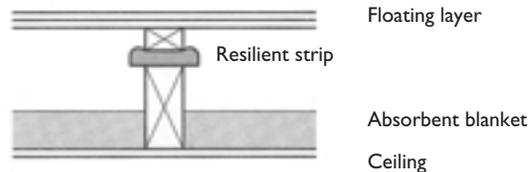
Floating layer of at least 18 mm thick timber or wood-based board with tongue and grooved edges and all joints glued and spot bonded to substrate of at least 19 mm thick plasterboard, or material with at least the same mass, nailed to 45 mm x 45 mm timber battens placed over the joists. Resilient strip of at least 25 mm thick mineral fibre, density 80 - 140 kg/m<sup>3</sup> laid on joists.
