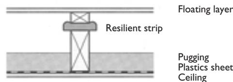
Floating layer of at least 18 mm thick timber or wood-based board with tongue and grooved edges and all joints glued and nailed to 45 mm x 45 mm timber battens on a resilient strip of at least 25 mm thick mineral fibre, density 80 - 140 kg/m<sup>3</sup> laid on joists.
