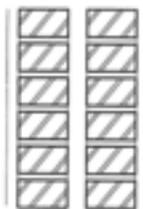
The width of the cavity should be at least 50 mm.
