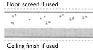
The average mass of the base (including the shuttering if it is solid concrete or metal, floor screed and any ceiling finish bonded to the shuttering) should be at least 220 kg/m<sup>2</sup>.
