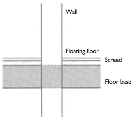
If the wall is a sound resisting or internal solid wall, with an average mass of less than 355 kg/m<sup>2</sup> (including any plaster finishes), the floor base including any structural screed should pass through.
