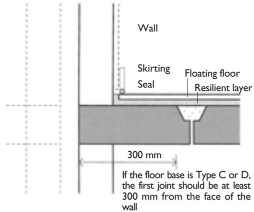
Carry the resilient layer up against the wall or isolate the floating floor.
