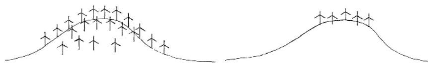
Fig 11: Wind farm is too spatially extensive relative to the scale of the hill.
